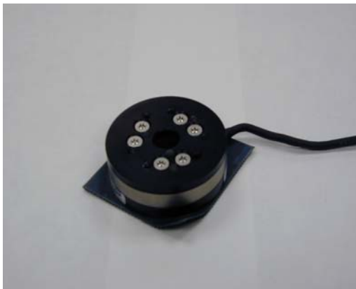
Figure 2 Three-dimensional force transducer used in the study
